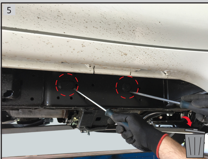
Right front bracket (B): On the chassis outer side remove the 2 caps
