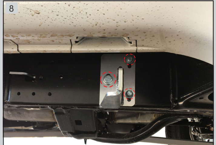
8 Connect bracket (B) to the chassis using hex bolt (L), spring washer (Q) and washer (O) to the spacer nut. Tighten hex bolt (K), spring washer (P) and washer (N)
