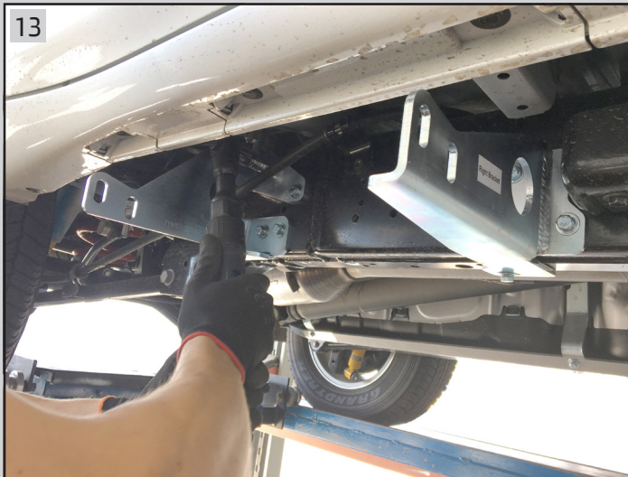
Tighten all 3 brackets bolts
