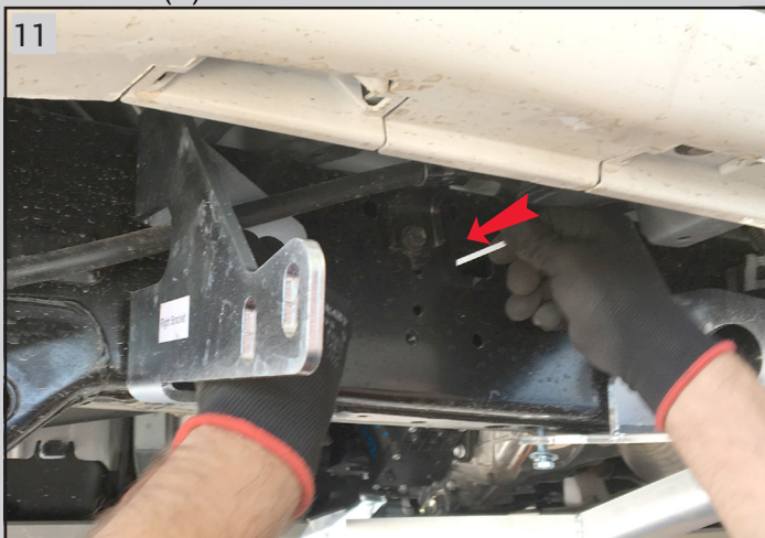
11 Place bracket (D). Insert 2 plates (J) through the chassis
