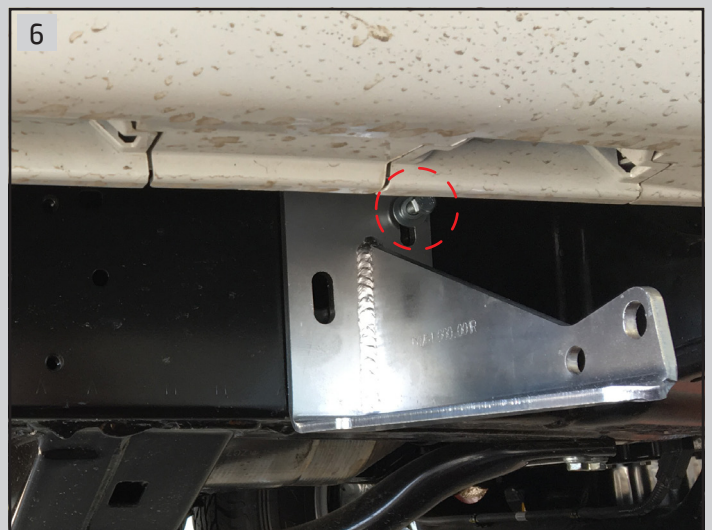
Place bracket (B) on chassis. Connect it to chassis using hex bolt (K), spring washer (P) and washer (N)
