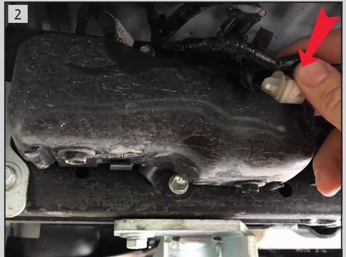
Insert the electrical outlet to the metal bracket as shown
