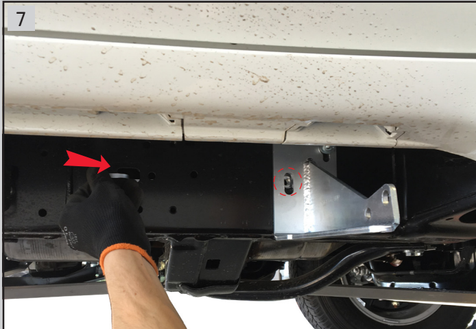
7 Insert spacer nut (H) through the hole into the chassis and align it to the hole of bracket (B)
