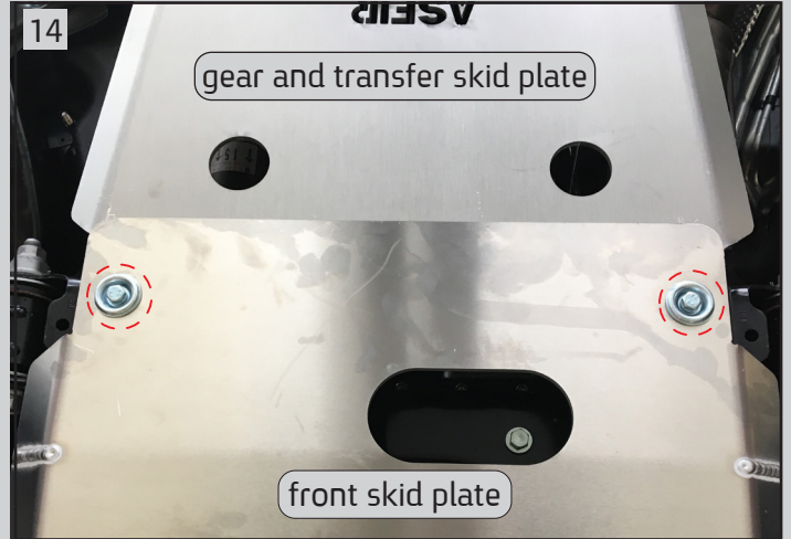
14 Use the spacer, pocket washer, spring washer and hex bolt from front skid plate to connect the front of skid plate (A) to chassis. Tighten all skid plate bolts
