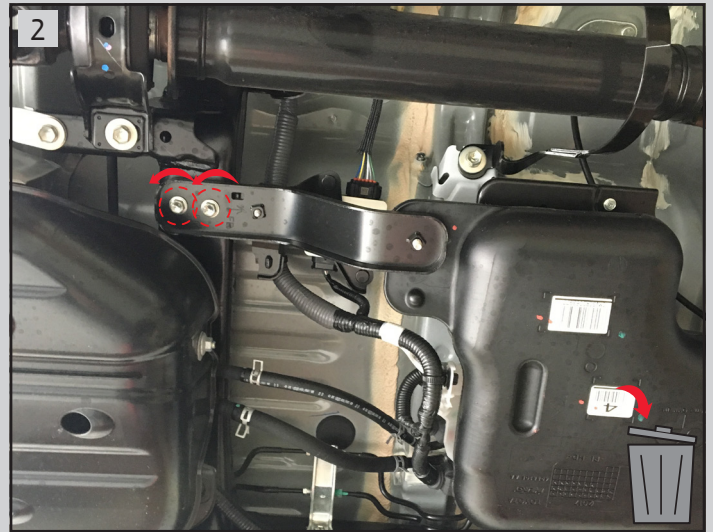
Remove 2 bolts of urea tank
