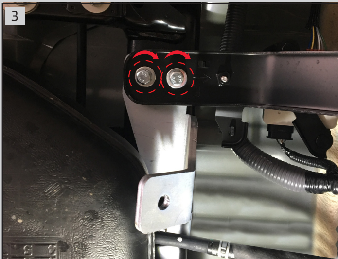
Place bracket (B) and tighten 2 hex bolts (D), spring washer (G) and washer (H) through bracket (B) and chassis
