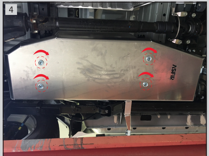
Connect plate (A) using 4 original bolts with hex nut (F), pocket washer (C) to original screwing
