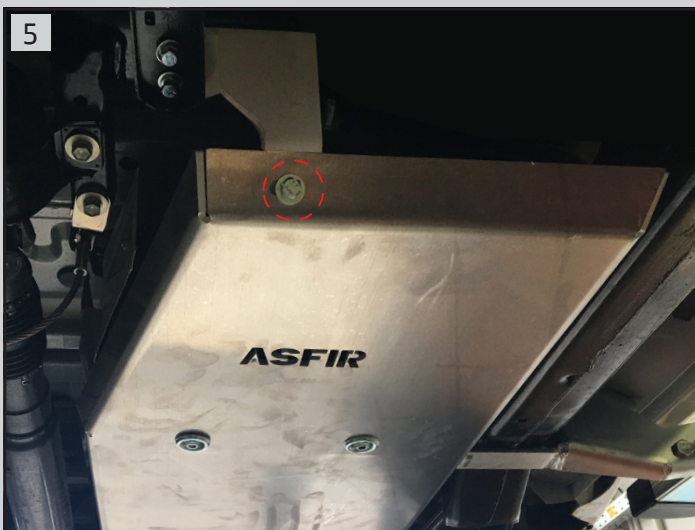
Connect plate (A) to bracket (B) using bolt (E), washer (H- on both sides of the plate) and hex nut (F)
