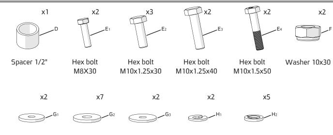
Washer 8x30 Washer 10x30 Washer 10x40 Spring washer 8 Spring washer 10
