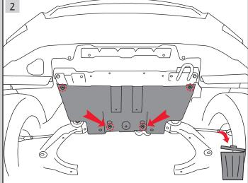
After removing the original skid plate reassemble the bolts (as marked)
