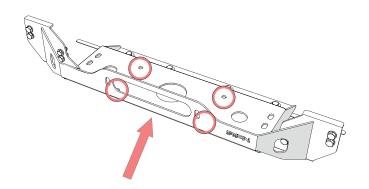
Once that is done, fit the Winch you have to be mounted using the marks in the red circles.
