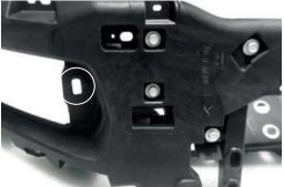
Take on Winch Bracket(1) and fit it on the vehicle.
