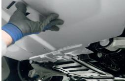
Then, go to the Plastic fenders, and loosen all the OEM\* Bolts of it.
