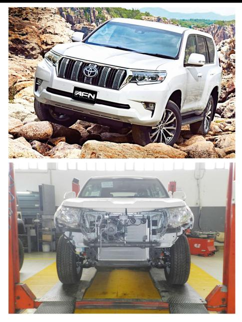
In our case, we also removed the grill of the vehicle in order to have more room to work. Be careful so you don't break the fasteners of the grill.
