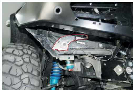
It's easier to cut plastic fender when the flaps are not installed.
