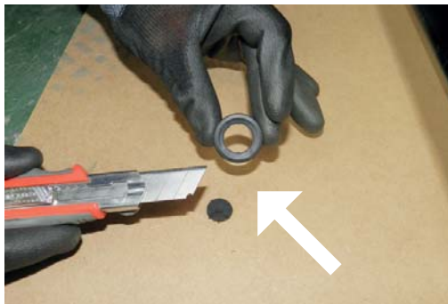
Only remove the inner circle if your vehicle has the Parking Sensor System installed.
